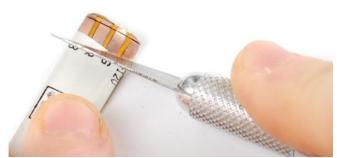
Scrape away the rubber to expose the copper pads.
